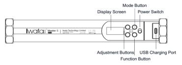
Slide the power switch to "green"/"red" to turn on/off the power.
